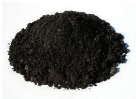
Figure 2-9: Dark brown or black color in soil usually indicates the soil has high organic content.
