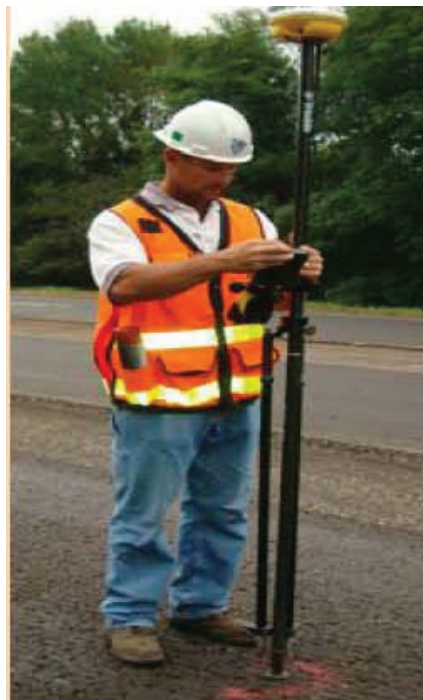
Figure 11-2: GPS rover being used to check surface elevation.
