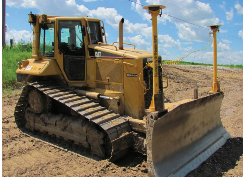
Figure 4-2: Dozer equipped with GPS
