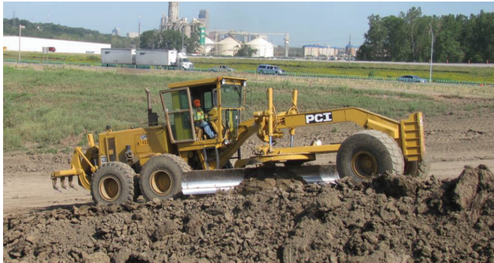
Figure 4-6: Motor grader (motor patrol)
