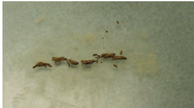
Figure 2-6: Test to determine plastic limit of soil.
