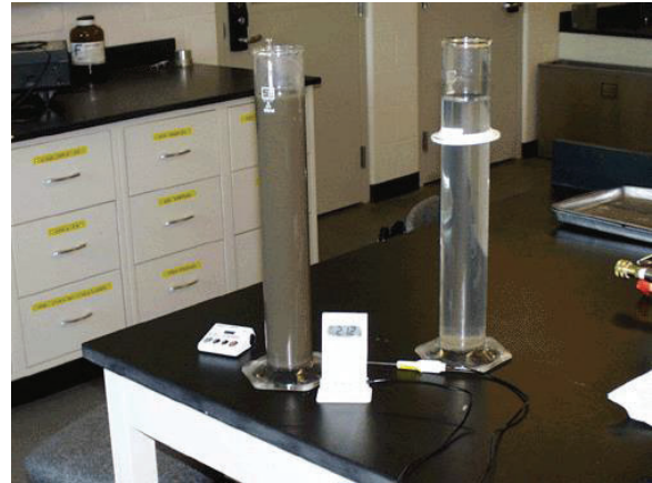
Figure 2-3: Hydrometer used to determine gradation of particles passing No. 200 sieve
