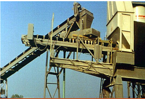
Slinger Feed Entry to Counter-Flow Drum-Mixer
