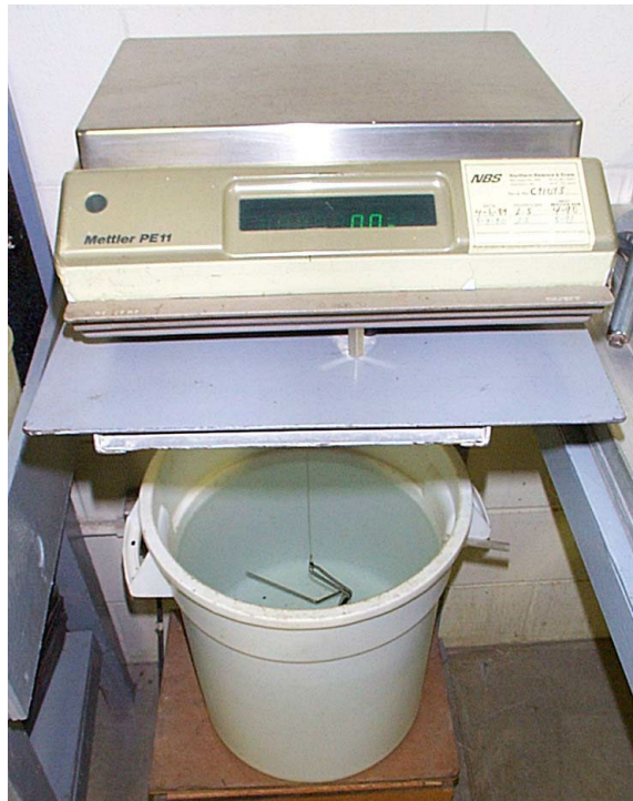
Balance, Sample Holder, and Water Container
