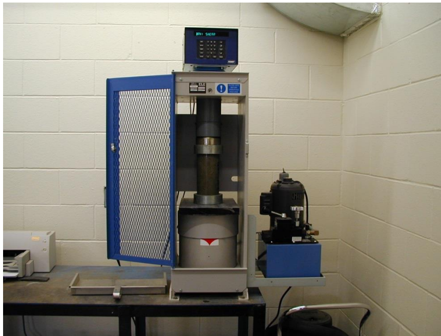
Figure 2. Compression Testing Machine
