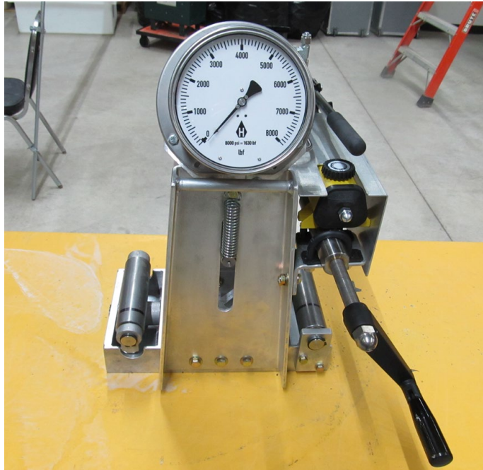
Figure 3. Hydraulic Testing Machine for Testing Four Inch Beams
