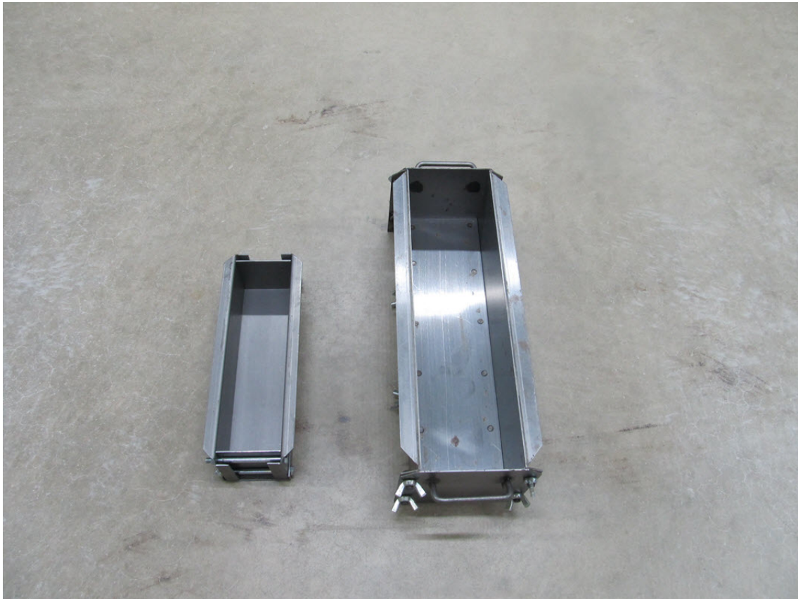
Concrete Beam Molds
