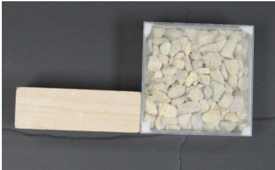
Figure 5-3 Absolute volume versus bulk volume of an aggregate
