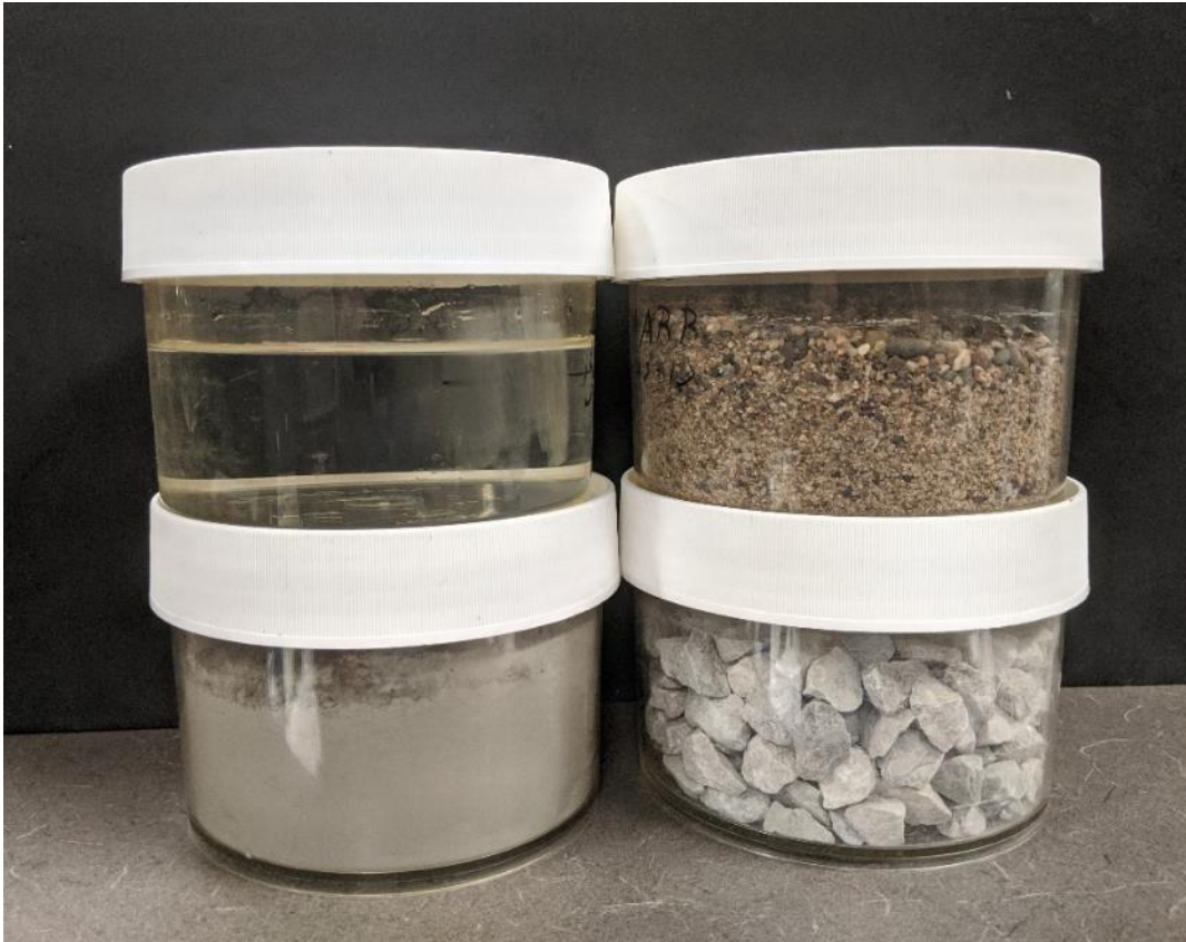
Figure 1-2 Composite materials of rock, sand, cement, and water
