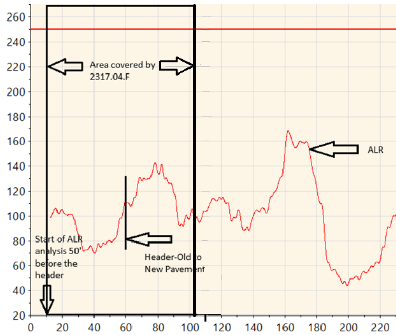
Figure 4-Area of Localized Roughness (ALR) at the beginning of a project. Same at the end of a project.
